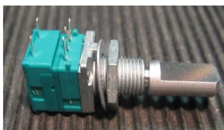
Type A, produced by DDM, is Conrad art.nr. 705594-89, which I have used for a long time already, and for which the PCB footprint was designed. It lacks a facility to screw it into a front plate. I only recently discovered type B in the Conrad catalog, art.nr. 700697-89. This switch from
